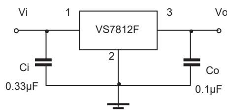
Note: Bypass capacitors are recommended for optimum stability and transient response and should be located as close as possible to the regulators.
